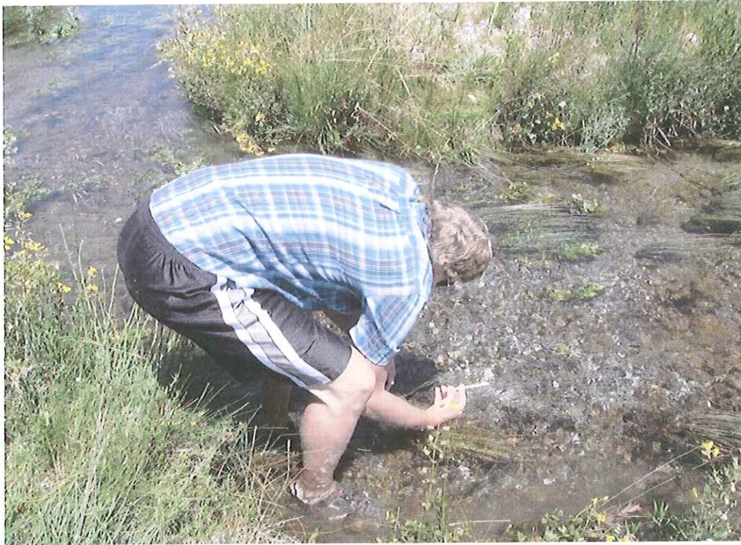
Illustration 6. Temperature readings were averaged from two thermometers that were placed in the middle of stream currents.
