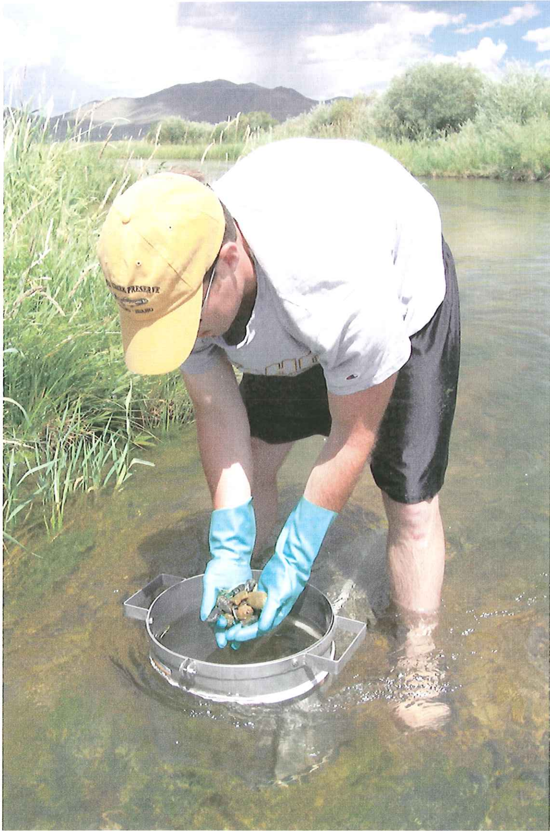
Illustration 8. A modified Hess sampler was used to collect benthic macroinvertebrates. All plant material and substrate were scrubbed and cleared of any insects.
