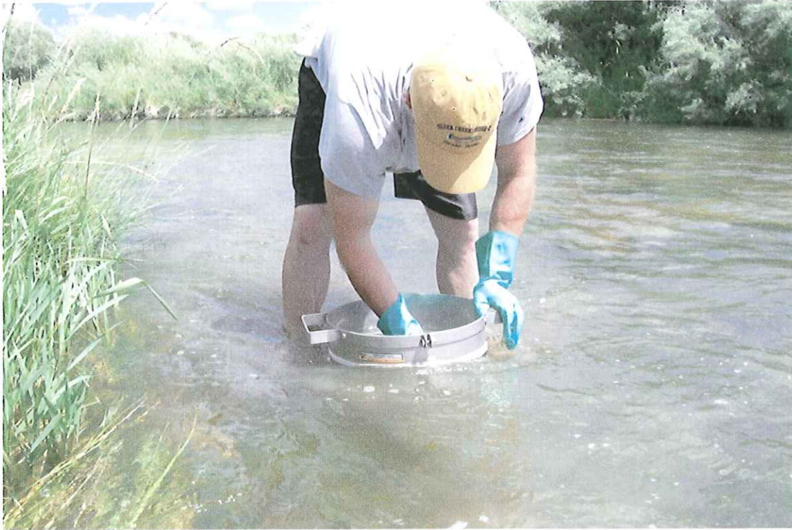
Illustration 10. Sample Site #1 has the presence of riffle like habitat. Sampling conditions here were suitable to use the Hess sampler without an extension tube.
