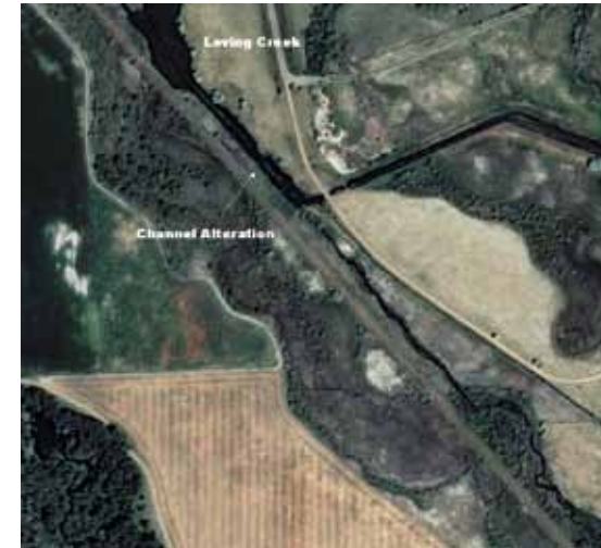
Channel alteration and straightening on Loving Creek above the diversion. The adjacent railroad grade and the canal diversion to the fish hatchery disconnected Loving Creek from its historic channel and floodplain.
