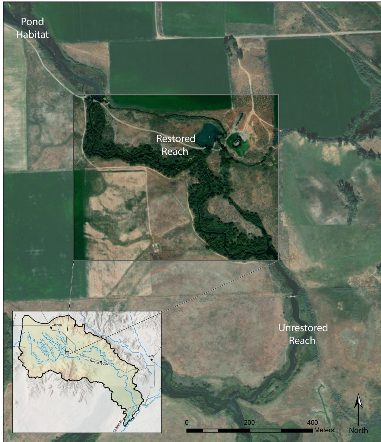
Figure 6-2. Example of Previously Restored Upper Subreach of Lower Loving Creek and Unrestored Lower Subreach of Lower Loving Creek
