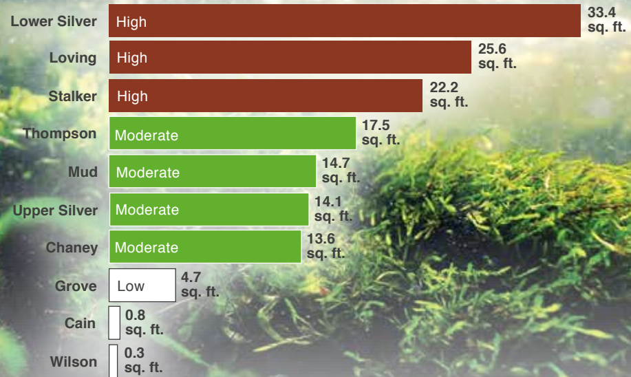
▲ Average Sediment Accumulated by Stream In 2011, sediment area was measured at 60 cross sections to estimate each stream's condition. Transects were averaged for each creek to categorize streams into high, medium and low. For example, the average area of sediments for all transects on Lower Silver is 33.4 square feet (sq. ft.).
